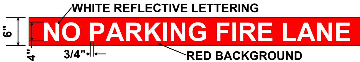
Figure 17 - Detailed fire lane striping design
