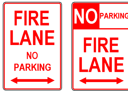
Figure 11 - Fire lane sign alternatives
