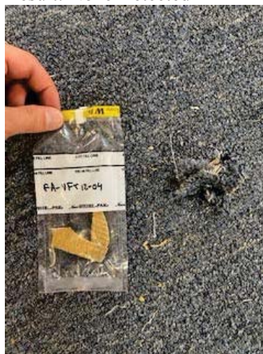
Sample: GA-VFT12-04 Result: 10% Chrysotile in tile
