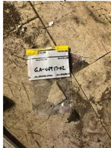
Sample: GA-VFT17-02 Result: 7% Chrysotile in black mastic
