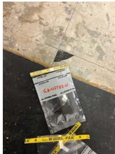
Sample: GA-VFT32-02 Result: 4% Chrysotile in tile
