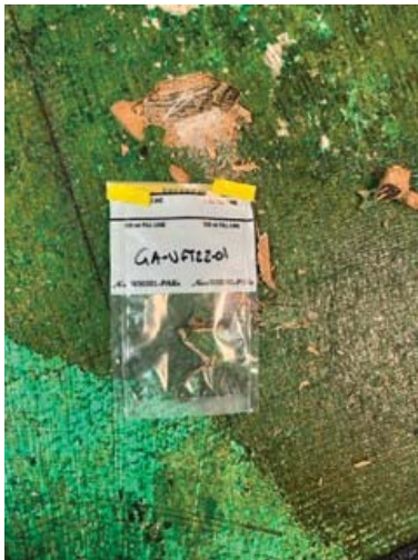
Sample: GA-VFT22-01 Result: 12% Chrysotile in tile
