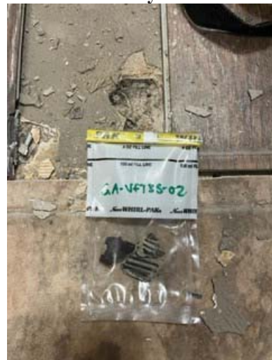
Sample: GA-VFT35-02 Result: 7% Chrysotile in tile
