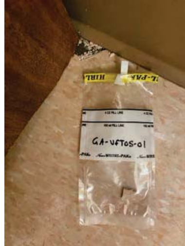
Sample: GA-VFT05-01 Result: None Detected 7% Chrysotile in black mastic
