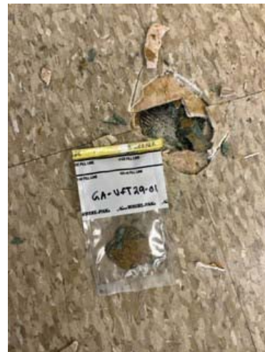
Sample: GA-VFT29-01 Result: 7% Chrysotile in tile
