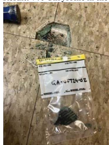
Sample: GA-VFT29-02 Result: 7% Chrysotile in tile
