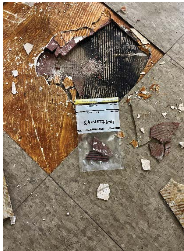
Sample: GA-VFT26-01 Result: 7% Chrysotile in tile
