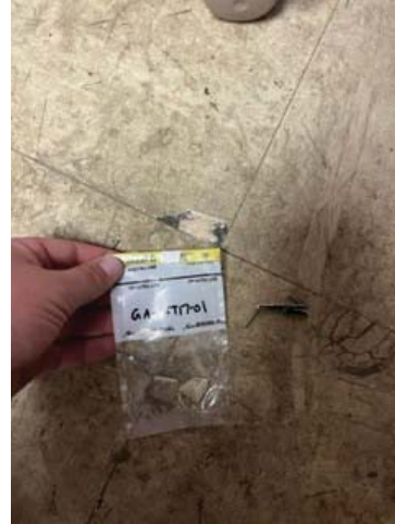
Sample: GA-VFT17-01 Result: 6% Chrysotile in black mastic
