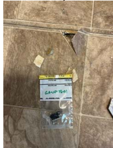
Sample: GA-VFT35-01 Result: 6% Chrysotile in tile
