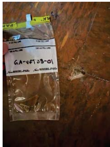
Sample: GA-VFT03-01 Result: None Detected 7% Chrysotile in black mastic
