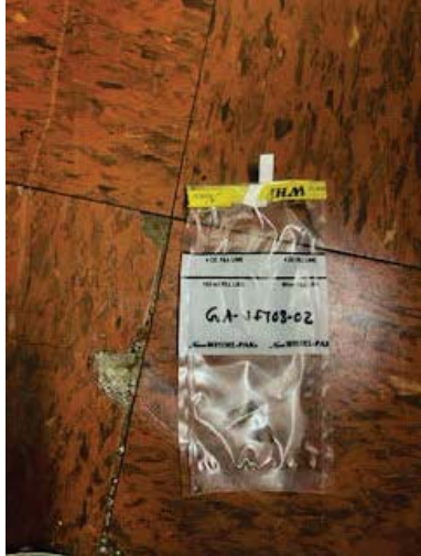
Sample: GA-VFT03-02 Result: None Detected 6% Chrysotile in black mastic
