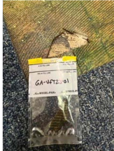
Sample: GA-VFT23-01 Result: 10% Chrysotile in tile
