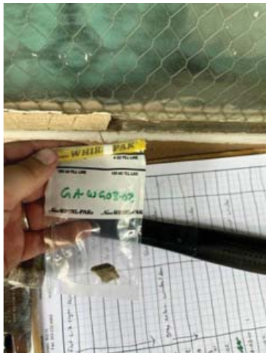
Sample: GA-WG03-02 Result: Trace Chrysotile
