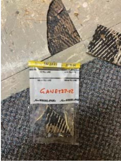
Sample: GA-VFT32-02 Result: 4% Chrysotile in tile
