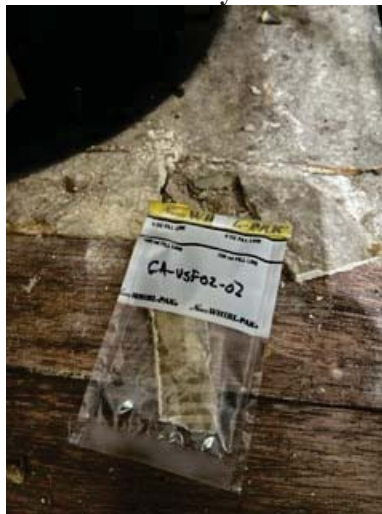
Sample: GA-VSF02-02 Result: 20% Chrysotile in backing
