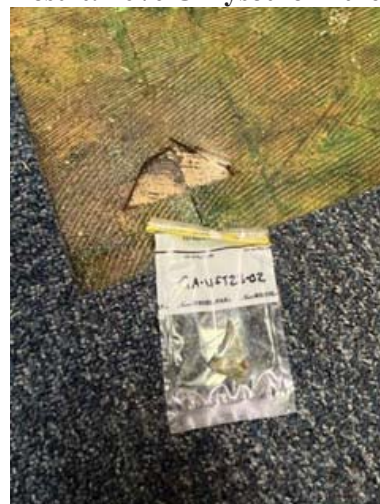
Sample: GA-VFT23-02 Result: 10% Chrysotile in tile
