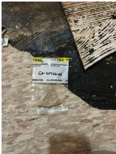
Sample: GA-VFT06-01 Result: None Detected 8% Chrysotile in black mastic
