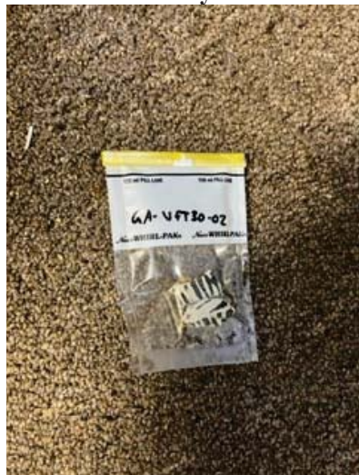
Sample: GA-VFT30-02 Result: 10% Chrysotile in tile
