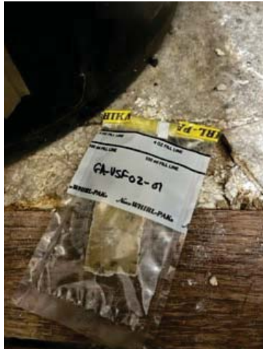
Sample: GA-VSF02-01 Result: 20% Chrysotile in backing
